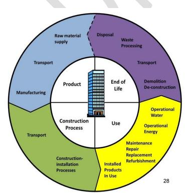
The illustration shows what comprises a typical building life cycle scope according to the new European standard *EN* 15978. It will be appreciated that whole building life cost assessment is a complicated process as buildings are comprised of multiple products, materials and services performing interdependently over a long and unpredictable service life.
