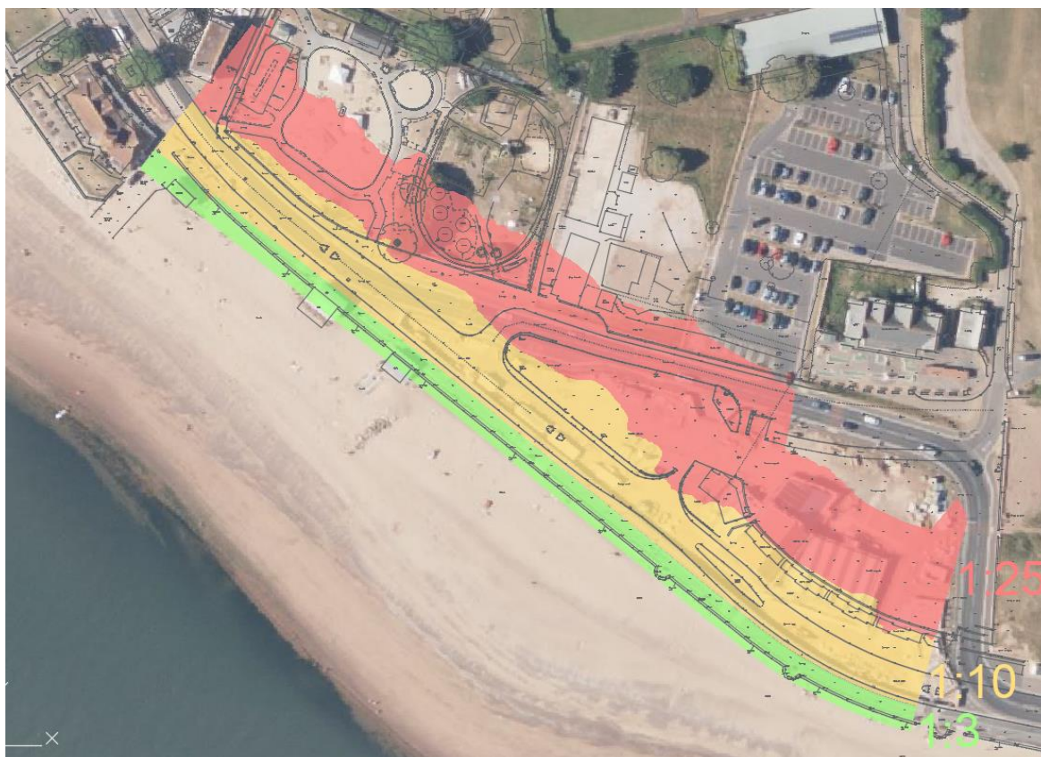
Image 6.1. Erosion map if seawall left to fail.
