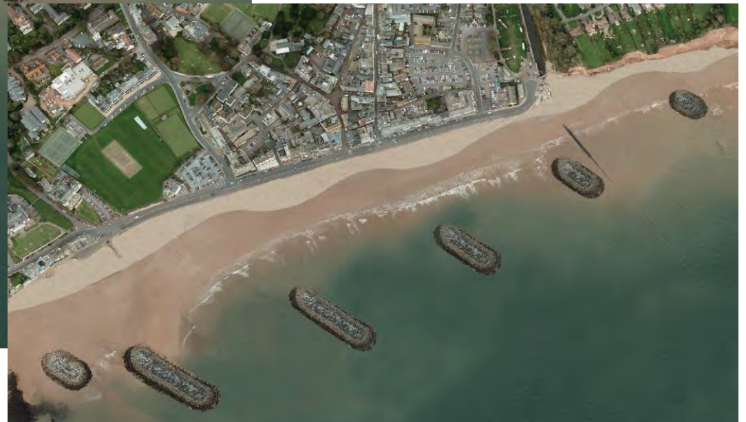
Illustration of how replacing groynes with more angled breakwaters could look.
